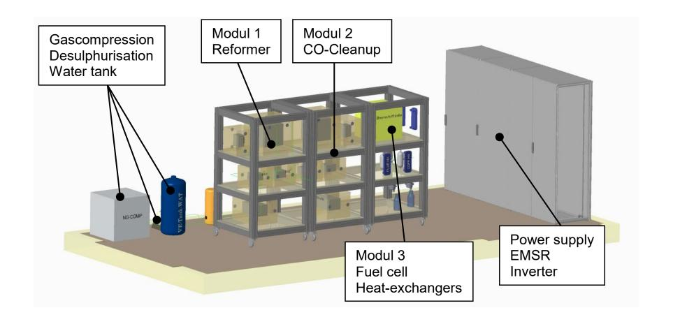
Complete system including fuel cell, BoPs and control system
