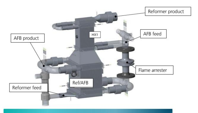
12,500 catalyst coated channels on each side
